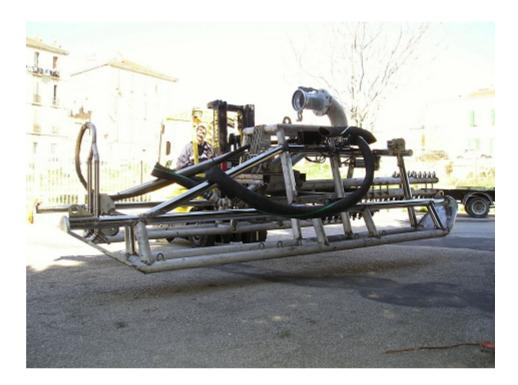
TJV 07 (Towed Jetting Vehicle) was designed and built for the post lay burial of power and telecom cables in shallow water.
